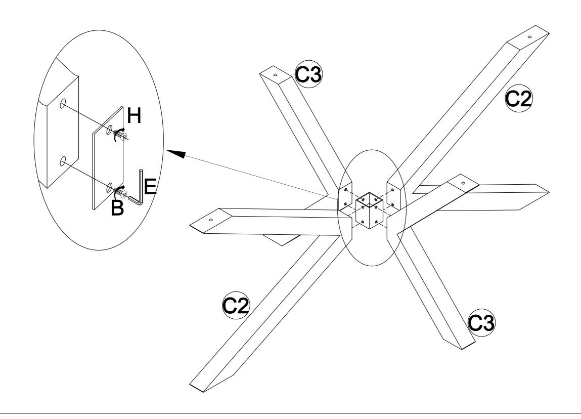
Step 2:Use Hex Key(E) to attach Leg(C2&C3) to the Panel(C1) with Bolt(A).
